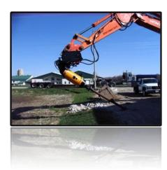
The positioning adapter plate is what enables the Pro-Dig T40K to function. **Oxford Hydraulics can** fabricate a plumbing system such as this one so that you can use your excavator to operate your machinery. The adapter plate is operating the Pro-Dig using a HITACHI 350LC excavator (left).
